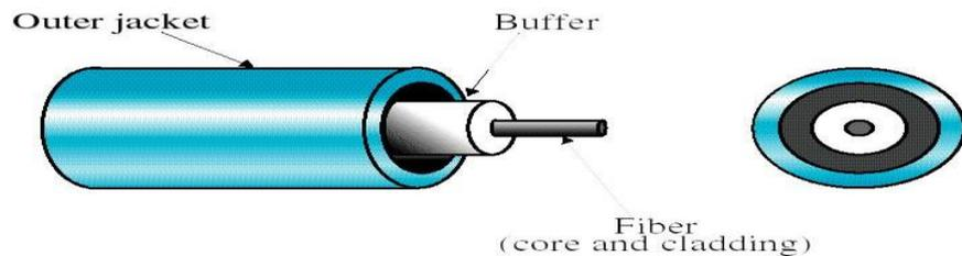
An optical fiber has an cylindrical shape and consists of 3 concentric section -
